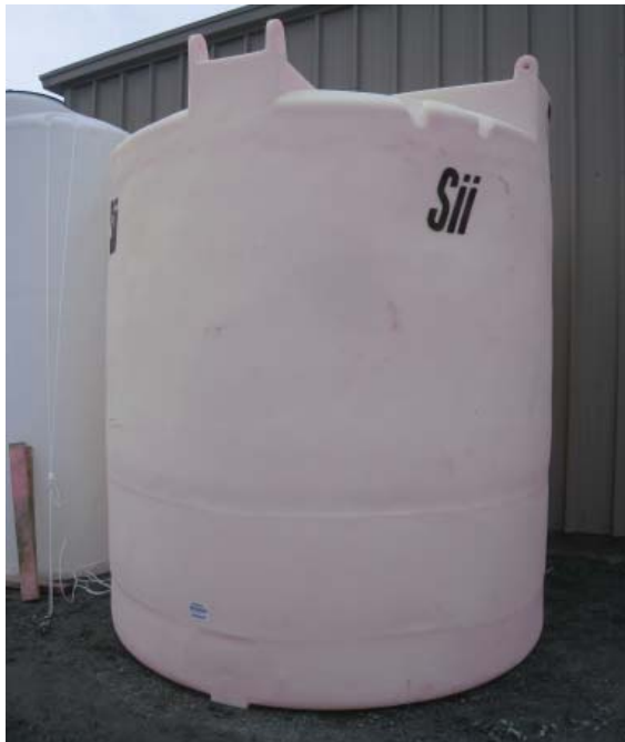
Pilot Plant Slow Sand Filter Tank
