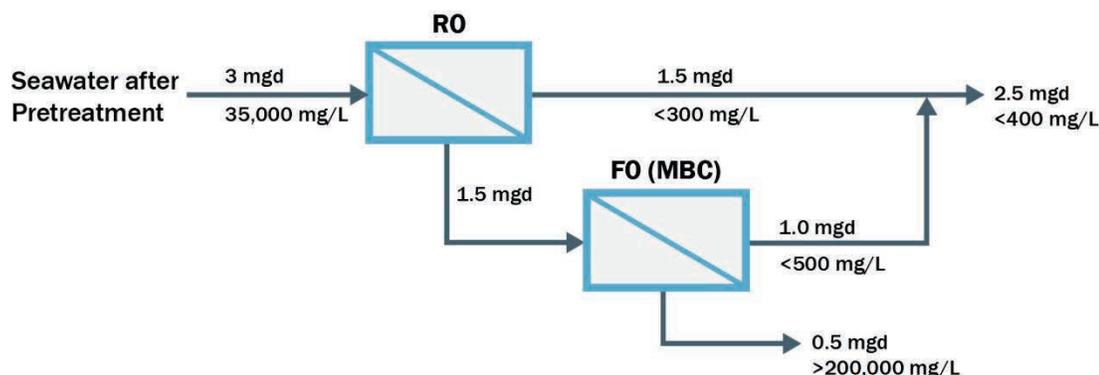
Figure 1. Water Balance Diagram with RO Brine Concentration by Forward Osmosis Membrane Brine Concentrator (MBC)
