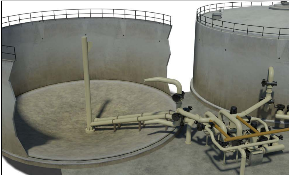
Figure 1: Typical Externally Pumped Digester Mixing System
