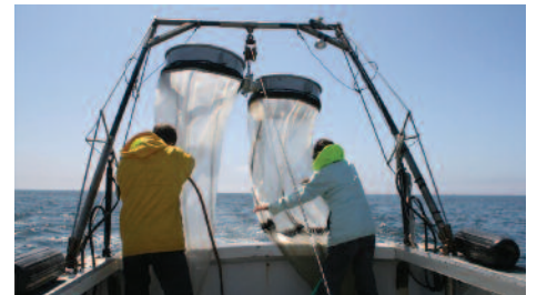
Paired plankton nets used to collect fish and shellfish larvae in the source water.
