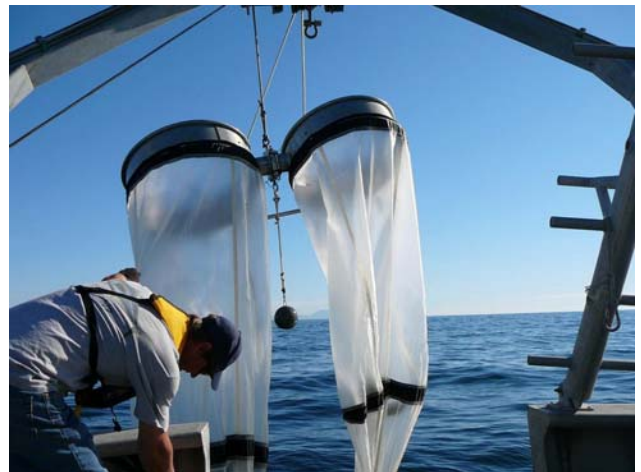
Figure 2-2. Paired plankton nets used for sampling (Tenera, 2010)
