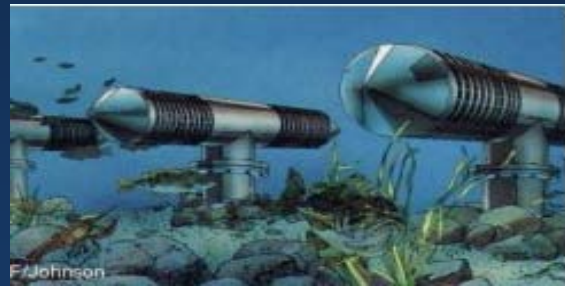
Passive screened intakes have very low intake velocities and small screen slot size which helps to minimize impacts.
