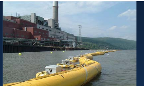
Aquatic Filter Barriers have worked well in lakes with minimal current forces on the fabric barrier.
